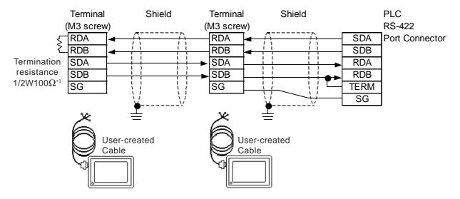
\*1 Please attach the termination resistor if needed. For the details, refer to the manual of the PLC.
